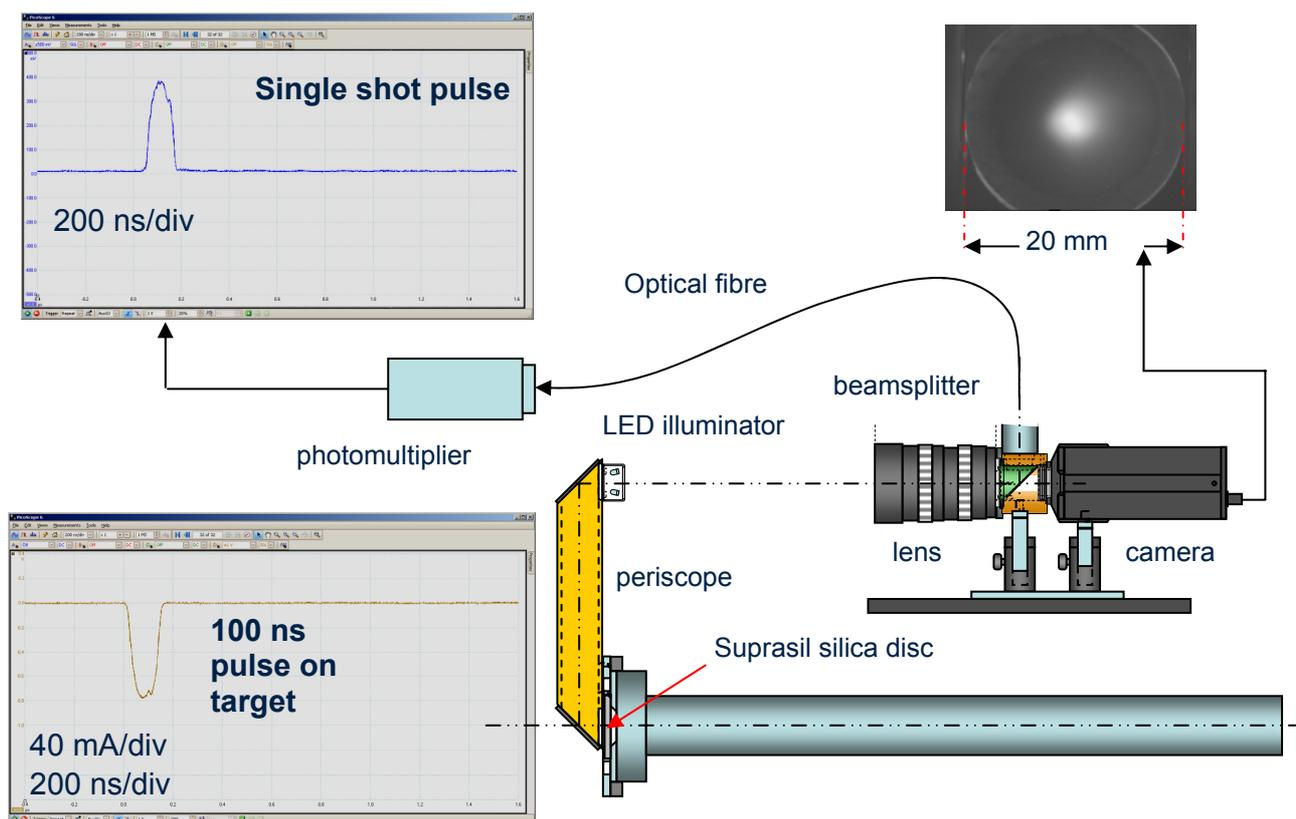
The lens/camera/beamsplitter can be rotated through +/- 90 degrees and the 'outputs' of any of the three beam lines can thus be monitored.
