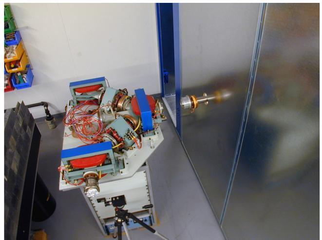
The immediate area outside of the beam end of the Faraday cage is dedicated to a beam switching magnet system. The rack below this is dedicated to DC magnet power supplies.
