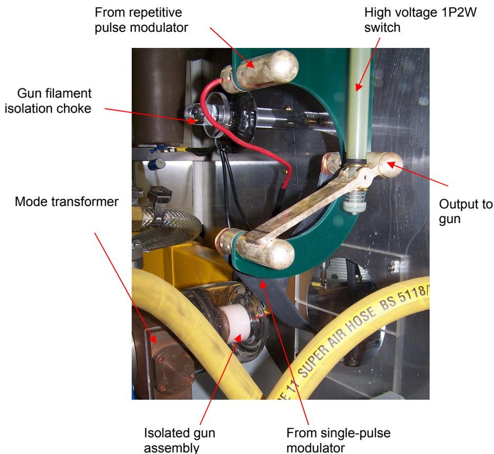
The gun modulator is based around somewhat dated, but effective thyatron switches (shown on the right); we had acquired several such switches over the years, and this approach was thus extremely cost-effective. Similarly, the output pulse transformer was ‘to hand’ and we were thus able to develop a novel type pulse generator to deliver many tens of kV at variable pulse widths.
