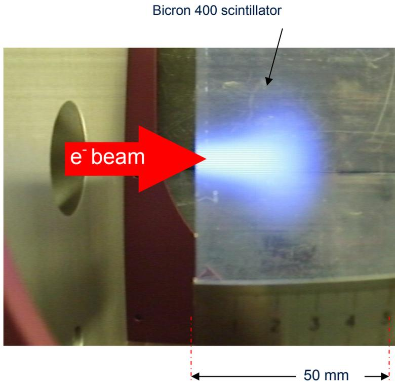
Electron beam luminescence in solid scintillator
