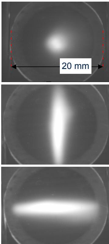
Beam shape control with quadrupole magnets
