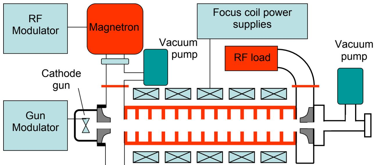
One of the features of our linac is that it is capable of producing single, variable width pulses on demand, in addition to the more usual repetitive pulses of  $\sim 4$   $\mu\text{s}$ . We achieve this by using a separate gun modulator. This is synchronized to the RF modulator and delivers a pulse to accelerate injected electrons during the much longer microwave pulse.
