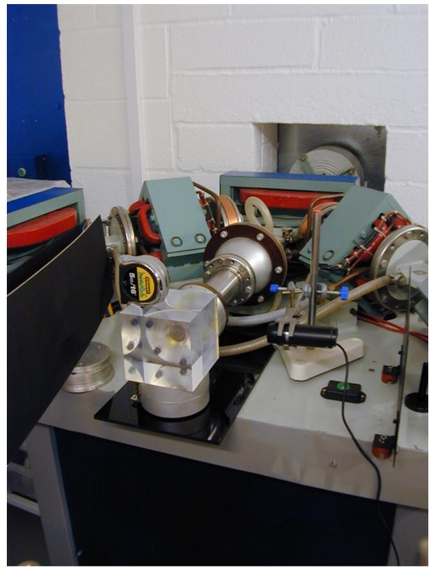
So now we had a neat Faraday cage enclosure with an accelerator inside it and a beam switching system outside the freshly painted shielding wall. We placed a scintillator block at the end of the beam line (right image) and turned everything on, hoping that it would work as expected. In reality of
