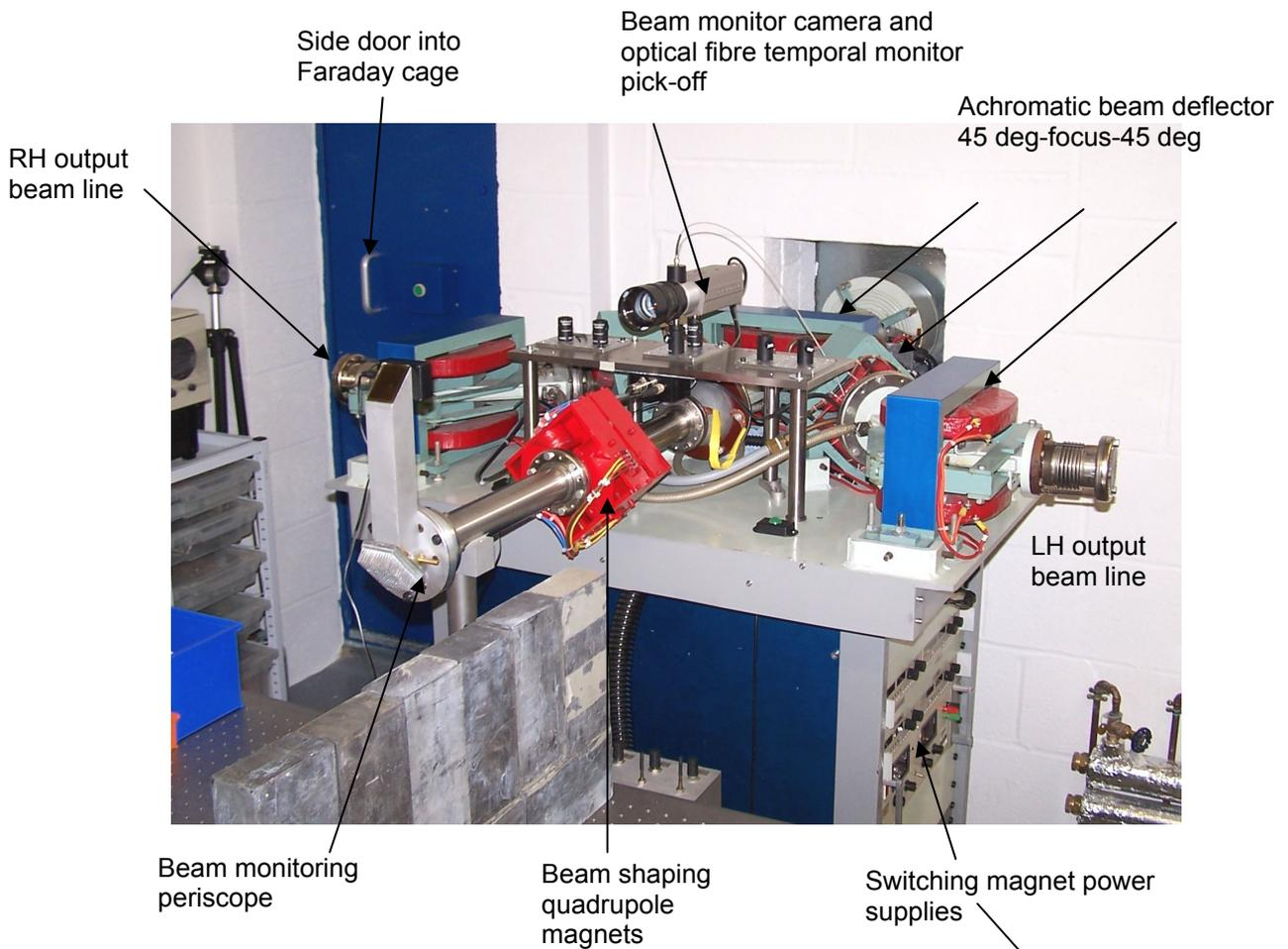
The beam deflection magnets and the beam monitoring system.
